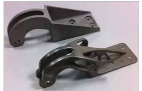
Fig. 1: Airbus A320 Nacelle Hinge Bracket (back) and the Optimised Design Produced by ALM (front)
