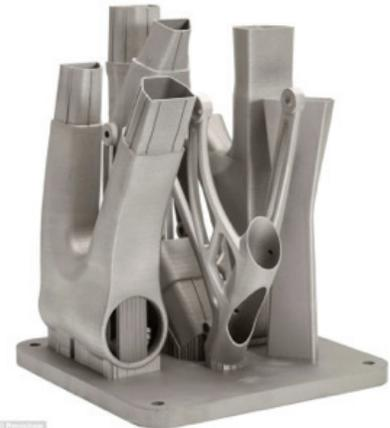
Bike frame components manufactured using additive manufacturing
